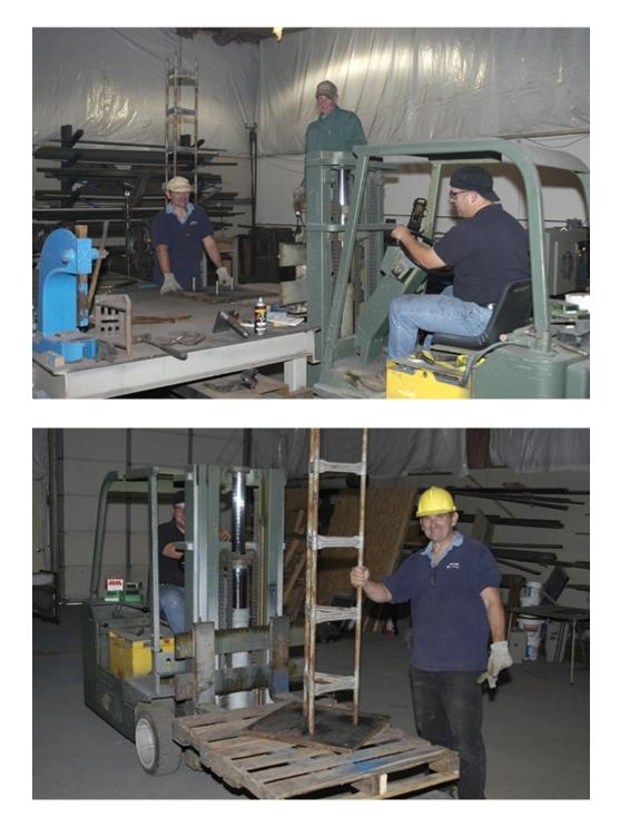
Joe, KC9FPD, shows off his tower base during loading operations. The top photo shows the base with the welded stubs. Below, Joe fits a short tower section to the stubs to check alignment.
