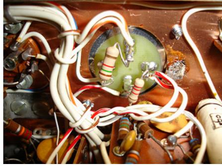
Bottom view of the new cap and resistors.
