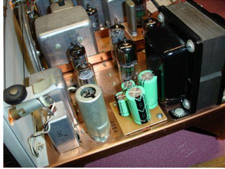
A right side view of the new filter capacitor.
