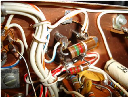
Bottom view of the old filter cap and resistors
