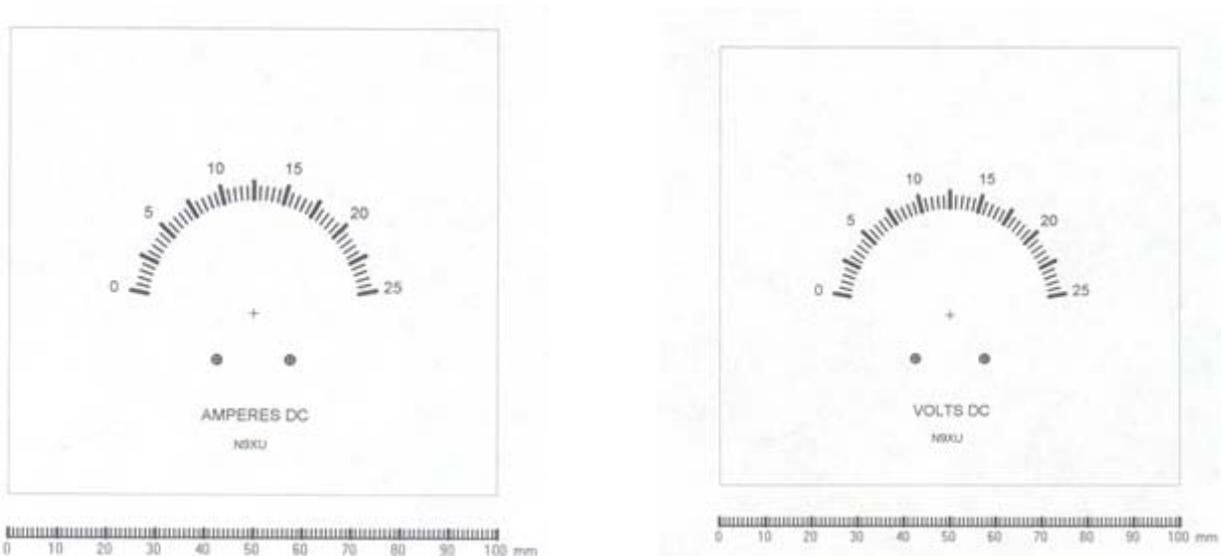
Samples of Dave's finished meter face graphics. These are scanned images, so they are not as crisp and sharp as the original items.
