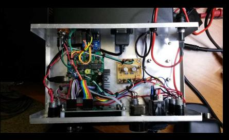
The controller reads the frequency of the radio and tunes the loop through the use of a stepper motor, which is connected to the capacitor. The capacitor can be a butterfly type or a vacuum variable.
