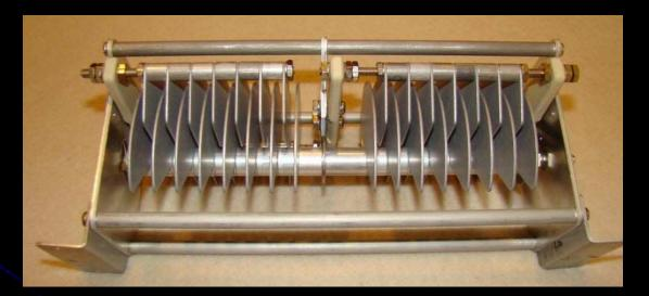
Large wide spaced split-stator style air variable capacitor
