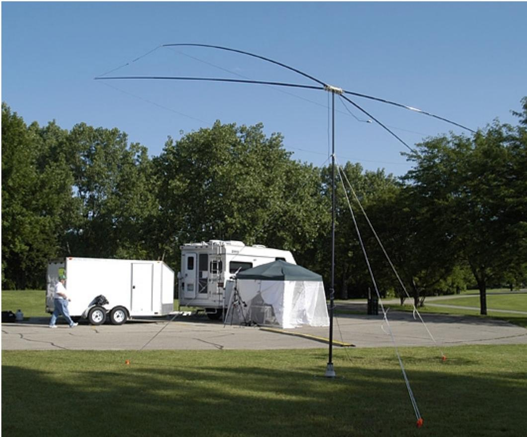
The 20 meter SSB station, with AH6EZ's stressed Moxon beam and portable rotating mast.
