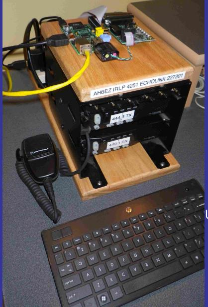
Duplexer, 15W load Motorola M1225 TX (5/25 watts) Motorola M1225 RX
