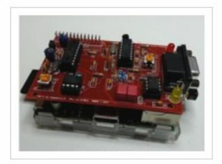
TNC-Pi is a terminal node controller device, GPIO add-on board used by amateur radio operators to participate in AX.25 packet radio networks.
